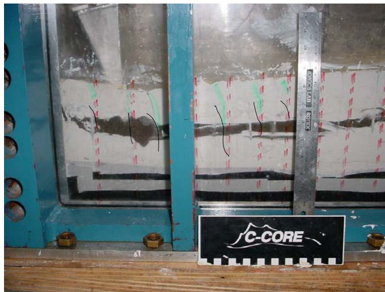
Figure 22: Photo of toe of slope after slope failure in test 2.
