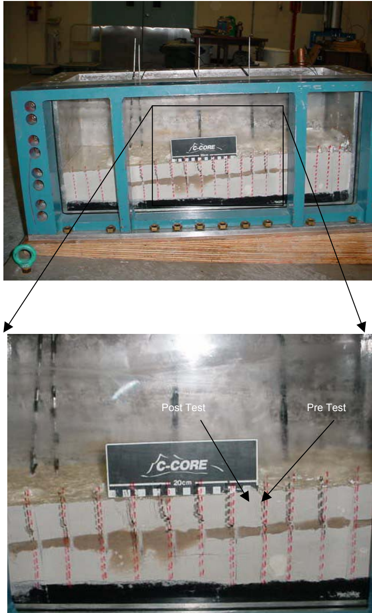
Figure 39: Observation of Slope Movement, Test 4.
