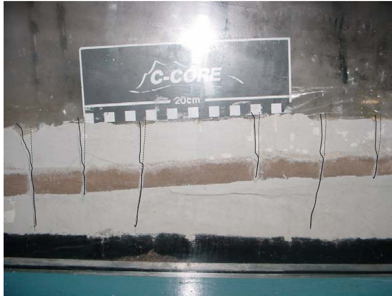
Figure 31: Slope Movement shown by Spaghetti Markers, Test 3
