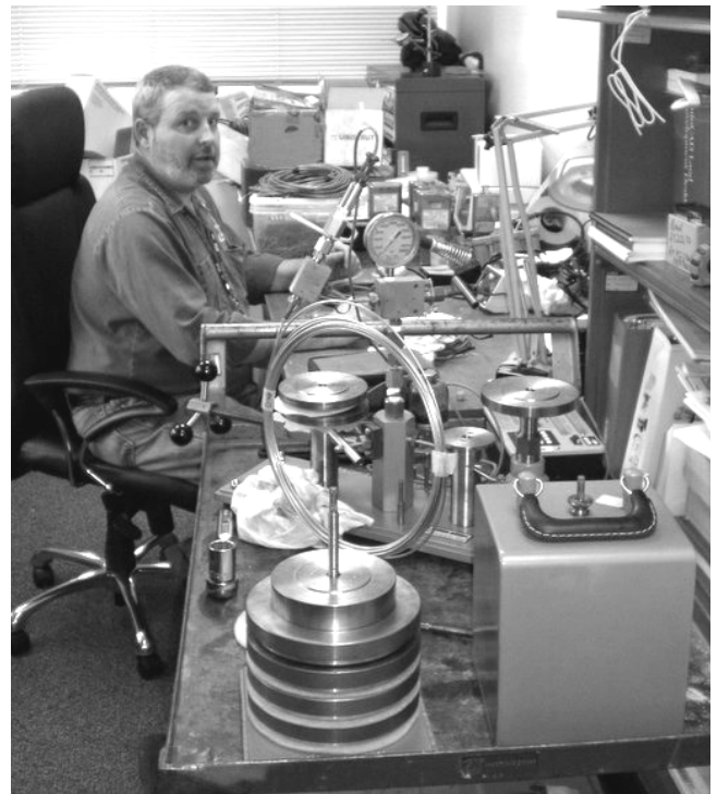
Figure 4. Borehole pressure cell transducers being calibrated in the laboratory using a dead-weight testing unit.
