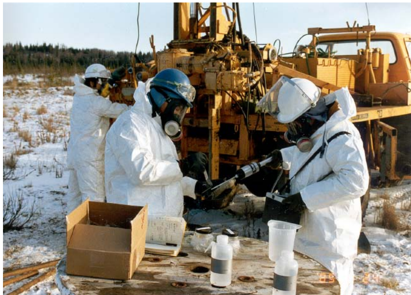
Over 1,000 soil samples were collected in association with the extensive PCB remediation efforts at Swanson River Field. USFWS Photo by Robert A. Richey.
