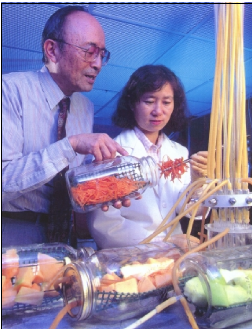
Food technologist Alley Watada (left) and horticulturist Ling Qi, who is visiting from China, prepare shredded carrots and other fresh-cut produce for automated measurement of respiration rate and ethylene production at the USDA-ARS Horticultural Crops Quality Laboratory in Beltsville, MD. (K7514-7)
