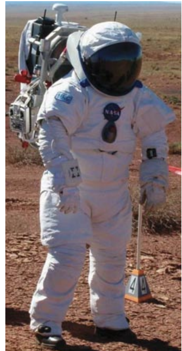
In 2004, ILC Dover, Inc.'s new I-Suit, an extra vehicular activity space suit, was tested in Meteor Crater, Arizona.
