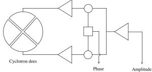
Figure 1: Block diagram of the modified RF system
