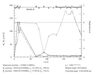
Figure 2: The IR and one FMC module of the 250 GeV isochronous *demo* muon collider lattice in the RHIC tunnel.
