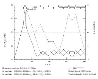
Figure 1: Isochronous RHIC lattice-IR with one FMC module.
