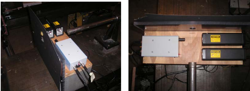
FIGURE 5. INITIAL VELOCITY MEASUREMENT SYSTEM (The photodiodes and their accompanying circuit are within the gray box.)
