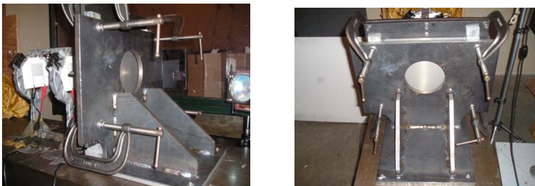
FIGURE 7. TARGET HOLDER WITH THE TARGET MOUNT ATTACHED
