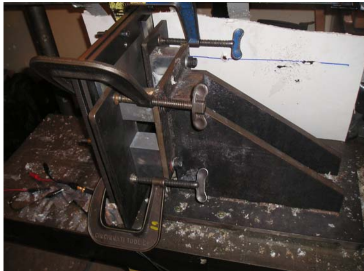
FIGURE 14. TARGET HOLDER ATTACHED TO THE TARGET MOUNT USED IN THE POWDER GUN SETUP
