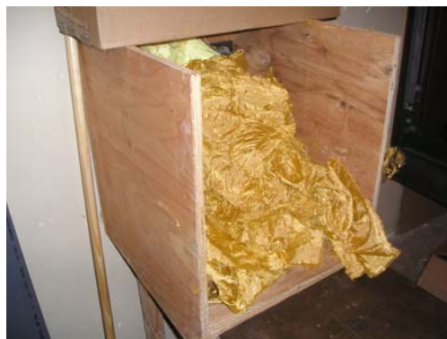
FIGURE 10. CATCHER BOX AT THE END OF THE GAS GUN
