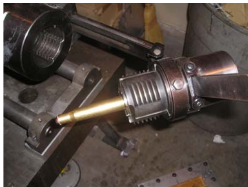
FIGURE 20. SHELL BEING LOADED INTO THE BREECH OF THE POWDER GUN
