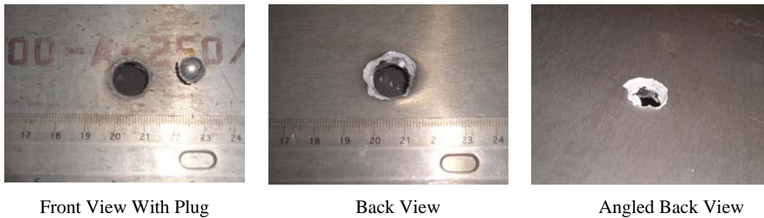
FIGURE 41. PLATE WITH AN INITIAL PROJECTILE VELOCITY OF 1875 ft/s
