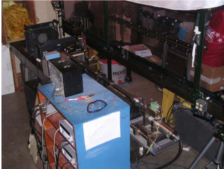
FIGURE 1. ANGLED VIEW OF THE GAS GUN SETUP USED FOR MOST OF THE TESTS
