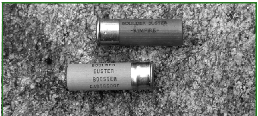
Figure 14—The Boulder Buster cartridge resembles a 12-gauge shotgun shell, but cannot be chambered in a shotgun.
