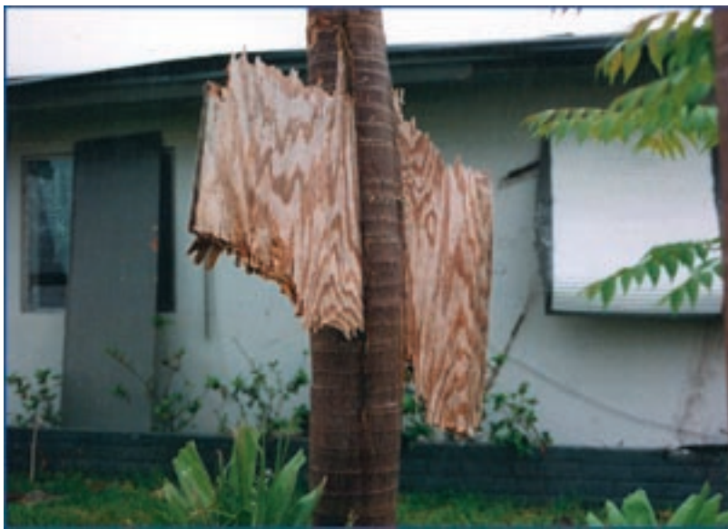
Palm tree pierced by plywood missile, Hurricane Andrew
