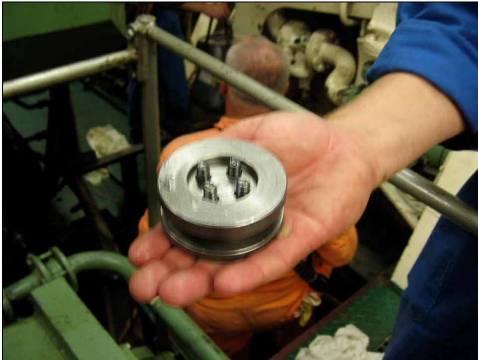
Figure 11: Demounted double sheave from the OD box
