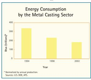
Most of the energy use in the metal casting sector (approximately 55% of total energy costs) can be attributed to the melting of metals, but moldmaking and coremaking also utilize significant amounts of energy. Opportunities to improve energy efficiency include updating old gas-fired equipment and substituting water for lubricant to cool heated die surfaces. 10
