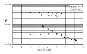
Figure 5: Q o vs. E<sub>acc</sub> at SHI-3 cavity.
