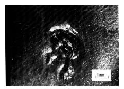
Figure 6: Equator defect found on SHI-3.
