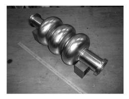
Figure 7: Overall view of 3 cell-cavity.
