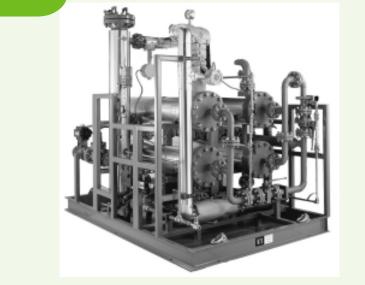
$\mathbf{M}$ embrane separation unit used in the reactor system to produce 95 percent pure isobutane.
