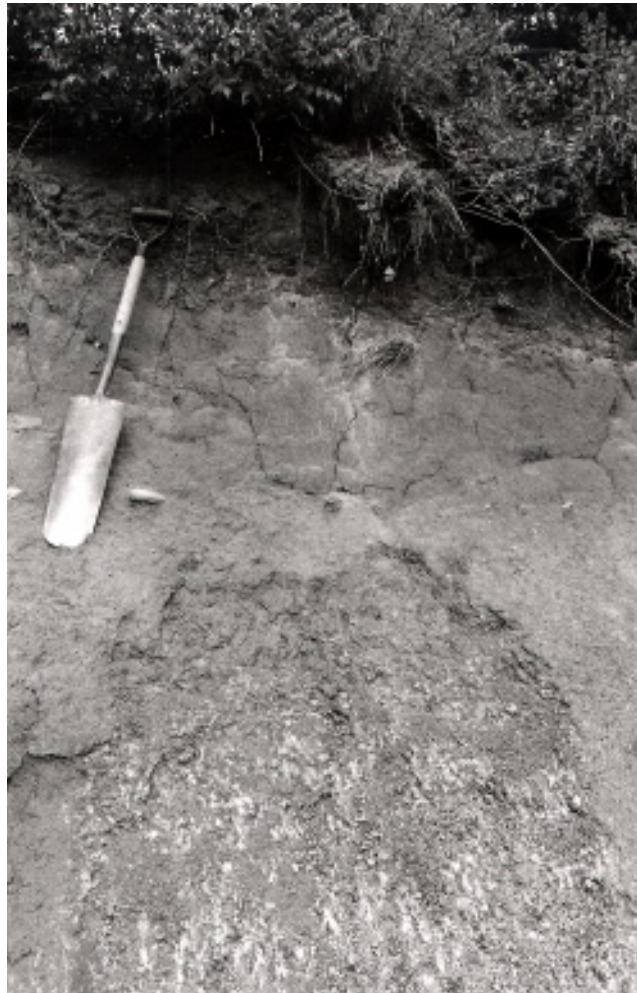
Figure 8. —Road cut in an area of Masada fine sandy loam, 2 to 6 percent slopes, showing a stone line at about 48 inches. This indicates that the river terrace deposits in which Masada formed covered an older landscape.
