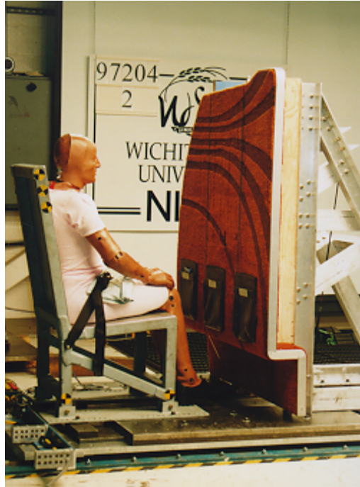
FIGURE 6. SETUP FOR CABIN CLASS DIVIDER PANEL TEST
