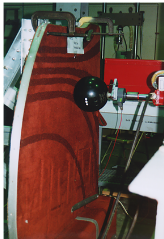
FIGURE 1. STATIC TEST SETUP FOR THE CABIN CLASS DIVIDER
