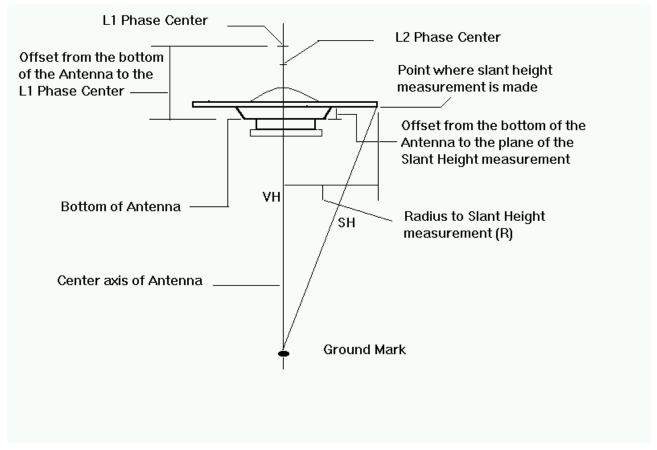
Radius to Slant Height Measurement (R): This is the horizontal distance from the vertical center axis of the antenna to the point where the slant height measurement (SH) is made.
