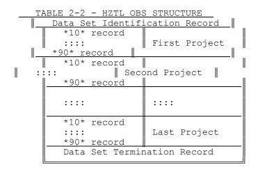
A horizontal control survey project is defined as a unit of field work containing a number of survey points (control points and peripheral points - see Chapter 1) which are connected by observations - horizontal directions, horizontal angles, vertical angles, distance measurements, and/or Global Positioning System (GPS) phase measurements. When coded as a part of an HZTL OBS data set, a project is a block of records comprising record groups arranged in the following order:
