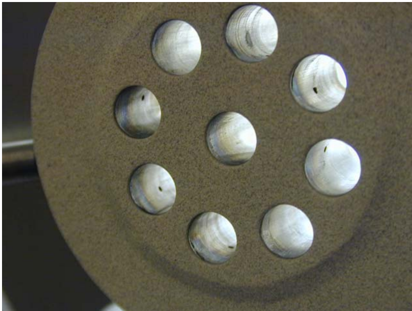
Fig. 1. NASA burner. a) Reactant inlet manifold (left) and windowed burner confinement section (right). b) Close up view of reactant inlet and H_2 radial injection holes.
