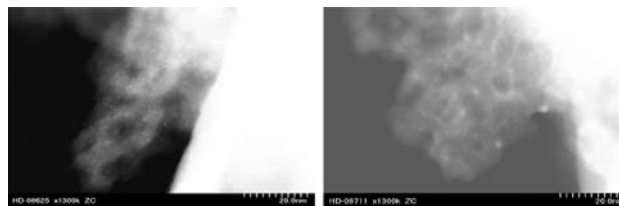
Figure 12. TEM of fresh and rich aged (500°C, 4 h) 2%Pt-98%[10%CeO 2 -ZrO 2 -90%(2%La 2 O 3 -98%BaO.6Al 2 O 3 )].
