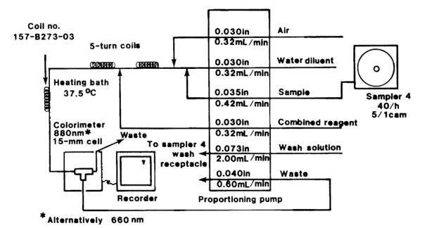
Figure 1. - Phosphorus, phosphomolybdate manifold
