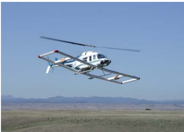
Figure 7. ORAGS-TEM system in transit near the Black Hills, South Dakota.
