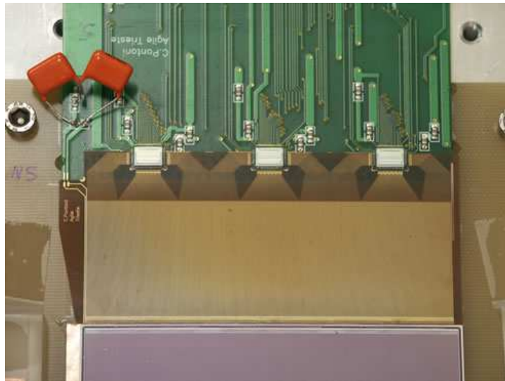
Figure 7.14: A magnification of the previous figure to show details of the read-out chips and the fan-out circuit.
