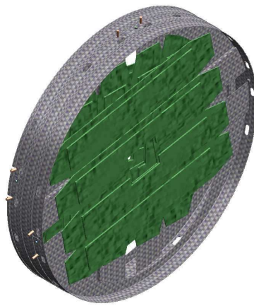
Figure 7.20: The support structure is such that the three views can be stacked to form a station. Reference pins guarantee a very precise relative alignment when assembling the components of the structure.
