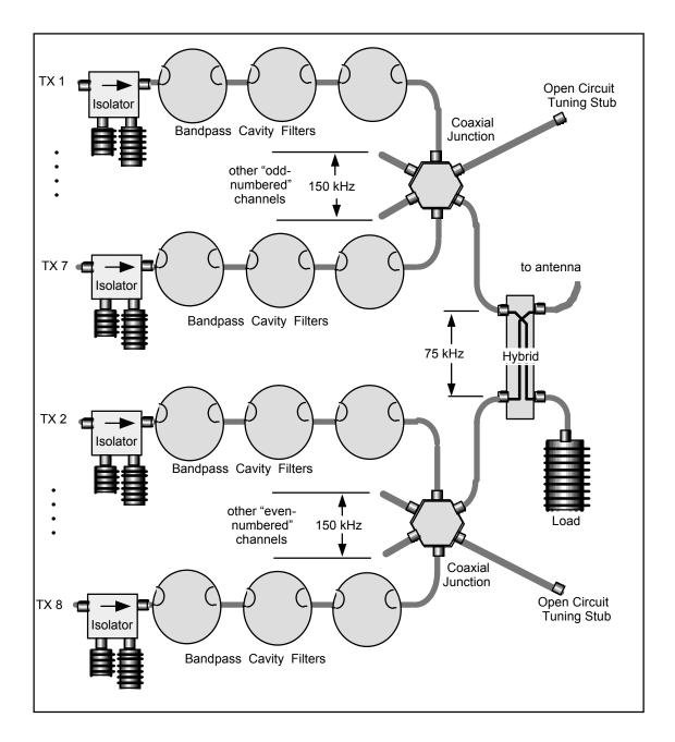
Figure 8. Composite cavity/hybrid combiner.
