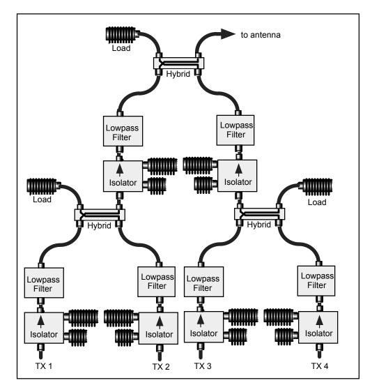
Figure 6. Four-channel transmitter hybrid-ferrite combiner.
