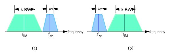
Figure 13. Bandwidth of intermodulation products: (a)  $f_{\rm rx} > f_{\rm IM}$ , (b)  $f_{\rm IM} > f_{\rm rx}$ . If the spectrum of the intermodulation product overlaps into the passband of a receiver, there is a potential for intermodulation interference.
