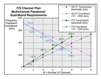
Figure 27. ITS band plan passband and guardband constraints.
