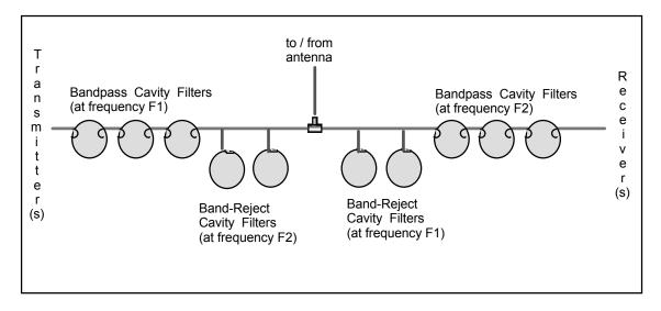
Figure 9. A duplexer constructed from parallel cavity filters.
