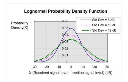
Figure 16. Probability distribution of the difference between the actual received signal level and the median signal level, for three standard deviations of the lognormal signal.
