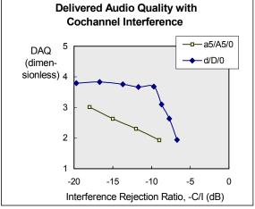
Figure 5. *Delivered audio quality* of demodulated speech signals under various interference conditions.
