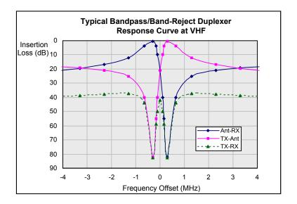
Figure 10. A typical frequency response for a duplexer. "Ant-RX" is the insertion loss between the antenna and receiver. "TX-Ant" is the insertion loss between the transmitter and antenna. "TX-RX" is the isolation between transmitter and receiver.
