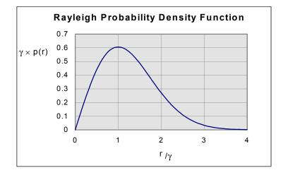
Figure 18. Normalized probability distribution of the magnitude of a Rayleigh-faded signal.
