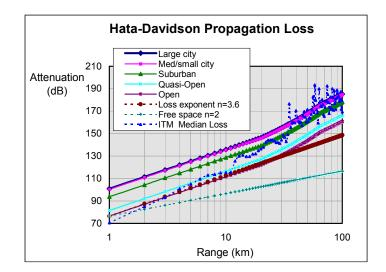
Figure 15. Hata-Davidson, exponential power loss, and ITM models of propagation loss for mobile communications at 161 MHz. Base station antenna height is 33 meters and mobile unit antenna height is 5 meters.
