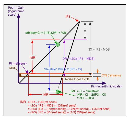
Figure 14. Amplifier intermodulation performance diagram.
