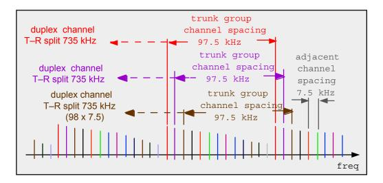
Figure 26. ITS band plan's channel spacing.
