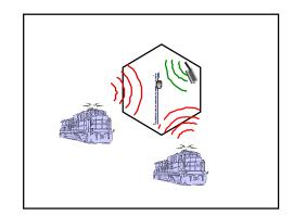
Figure 23. Portable-to-repeater situation: Two adjacentchannel mobiles near the boundaries of neighboring cells interfere with the reception of a desired signal from a lower-powered portable located within the target cell.
