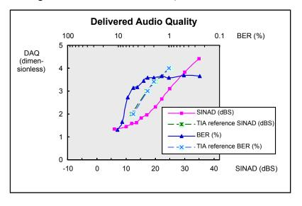
Figure 4. DAQ vs. SINAD and BER.
