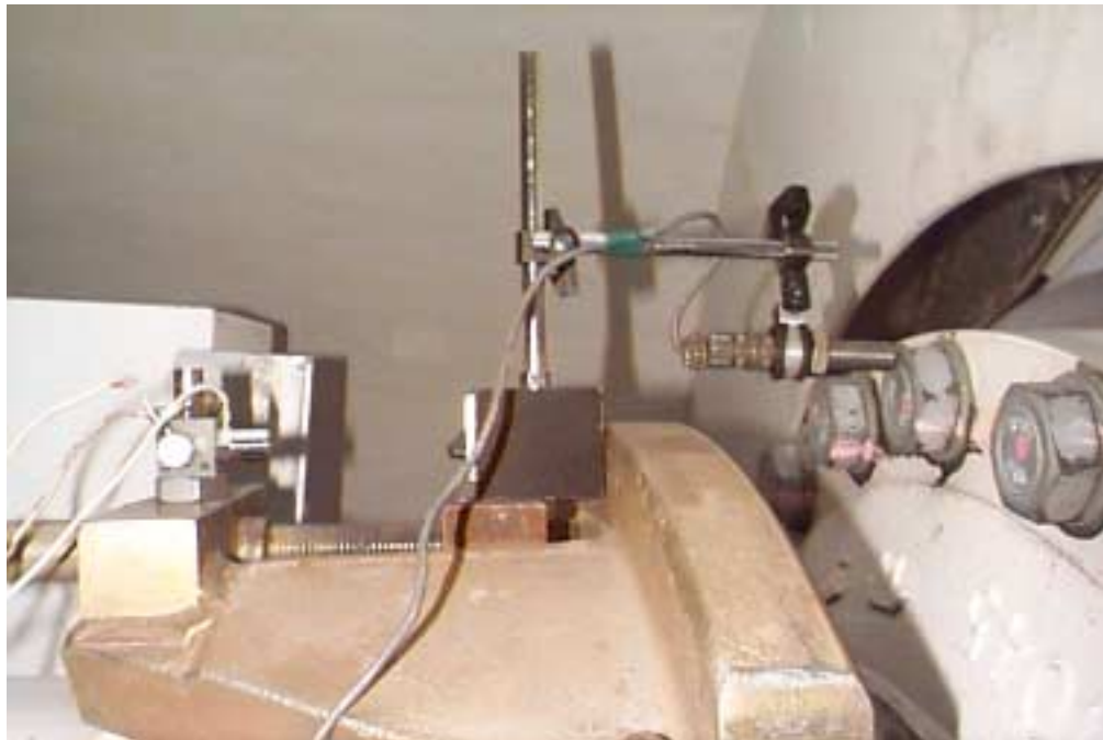
Figure 14. Rotor azimuth position and low-speed shaft sensors
