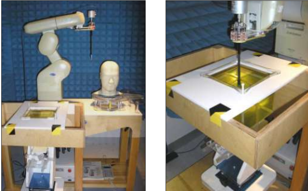
Figure 3: Principal components of the SAR measurement test bench
