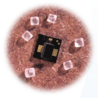
Verifying the desired atmosphere inside hermetic devices becomes much more difficult as package size decreases. Sandia researchers have developed methods and hardware to successfully sample and analyze the internal gas atmosphere of nanoliter packages (shown here with salt gains).
