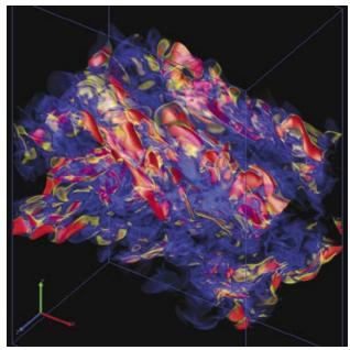
(Above) Sandia combustion researchers used a supercomputer at Lawrence Berkeley National Laboratory to perform the world's largest 3-D direct combustion simulation of a turbulent carbon monoxidehydrogen flame. The 10 terabytes of simulation data will be used to understand interactions to design more fuel-efficient, cleaner-burning engines.
