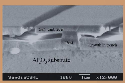
A scanning electron microscope image shows a cantilever epitaxy growth on top of the sapphire post. This Sandia-developed process for growing gallium nitride on an etched sapphire substrate may help light up the world with brighter green, blue, and even white high-efficiency light-emitting diodes.
