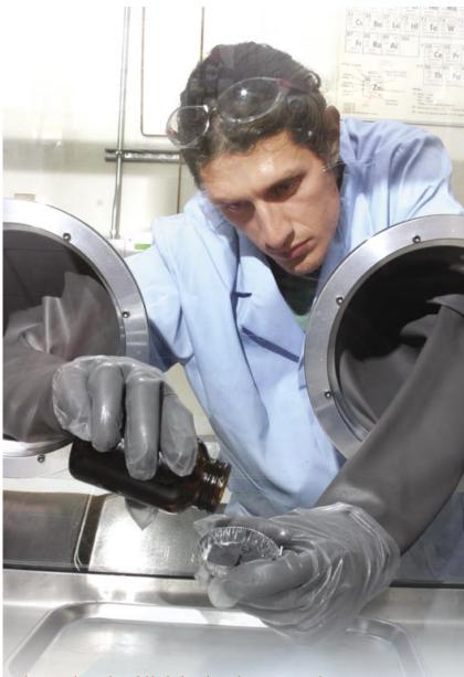
Sandia researcher with medal hydride sodium alanate, a material that can absorb and store hydrogen. General Motors and Sandia are partnering in a four-year, \$10 million project to design and test metal hydride materials for hydrogen storage.
