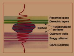
The laser cavity is fabricated with a space (a microfluidic channel) to allow the passage of whole cells or other biological material, as illustrated here.
