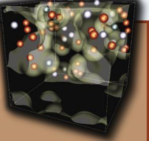
Quantum molecular dynamics simulation showing the atomic nuclei and an electron density iso-surface for stainless steel at high energy density. These simulations are being used to calculate the electrical and thermodynamic properties of stainless steel and other materials under the extreme current densities found on the Z machine. SANDIA NATIONAL LABORATORIES
