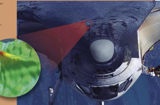
Extruding gap filler shown as LDRI data (in circle) from Sandia sensor. (NASA photo)
