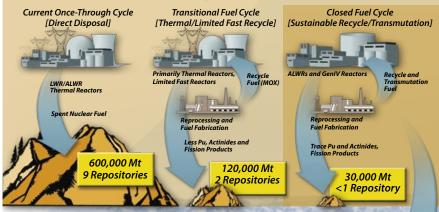
Improving the nuclear fuel cycle, first with recycling and then reprocessing, can dramatically minimize the tonnage of nuclear wastes destined for repository disposal.
