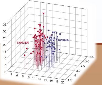
Transparent cells (or other biological material) have indexes of refraction that affect the laser output intensity, wavelength, and other characteristics. Different cell types produce different spectral characteristics from the laser, as this graph shows.
