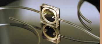
The BioCavity laser is based upon the Vertical Cavity Surface Emitting Laser, a Sandia-developed technology. A completed device with tubing to allow the flow-through of samples is shown here.
