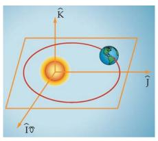
Figure 4.1.6-2. Heliocentric-ecliptic Coordinate System for Interplanetary Transfer. Origin—center of the Sun; fundamental plane—ecliptic plane (Earth's orbital plane around the Sun); principal direction—vernal equinox direction.
