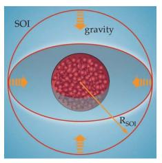
**Figure 4.1.6-6.** Sphere of Influence (SOI). A planet's SOI is the volume of space within which the planet's gravitational force dominates.
