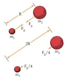
Figure 4.1.6-3. Newton's Law of Universal Gravitation. The force of attraction between any two masses is directly proportional to the product of their masses and inversely proportional to the square of the distance between them. Thus, if we double the distance between two objects, the gravitational force decreases to 1/4 the original amount.
