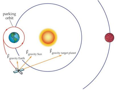
**Figure 4.1.6-4. Gravitational Forces on an Interplanetary Spacecraft.** Consider the forces on an interplanetary spacecraft as it makes its way from Earth to the target planet. We have the gravitational forces due to Earth, the Sun, and the target planet making it a four-body problem—Earth, Sun, target planet, and spacecraft.
