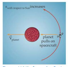
Figure 4.1.6-10. Spacecraft Passing behind a Planet. During a gravity-assist maneuver, a spacecraft's energy will increase with respect to the Sun if it passes behind the
