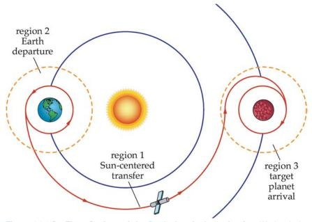
Figure 4.1.6-5. Three Regions of the Patched-conic Approximation. We break the trajectory for interplanetary transfer into three distinct regions in which the gravitational pull of only one body dominates the spacecraft's motion.
