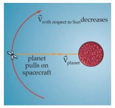
Figure 4.1.6-12. Spacecraft Passing in Front of a Planet. During a gravity-assist maneuver, a spacecraft's energy will decrease with respect to the Sun if it passes in front of the
