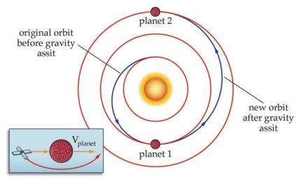
**Figure 4.1.6-11. Gravity Assist.** During a gravity assist, a planet pulls a spacecraft, changing its velocity with respect to the Sun and thus altering its orbit around the Sun. The planet's orbit also changes, but very little.
