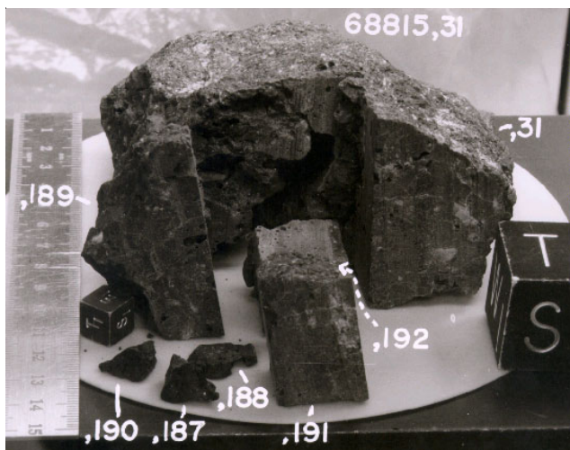
Figure 13: Group photo of saw cuts to produce column 68815,192 and ,191. NASA # S74-27981.
