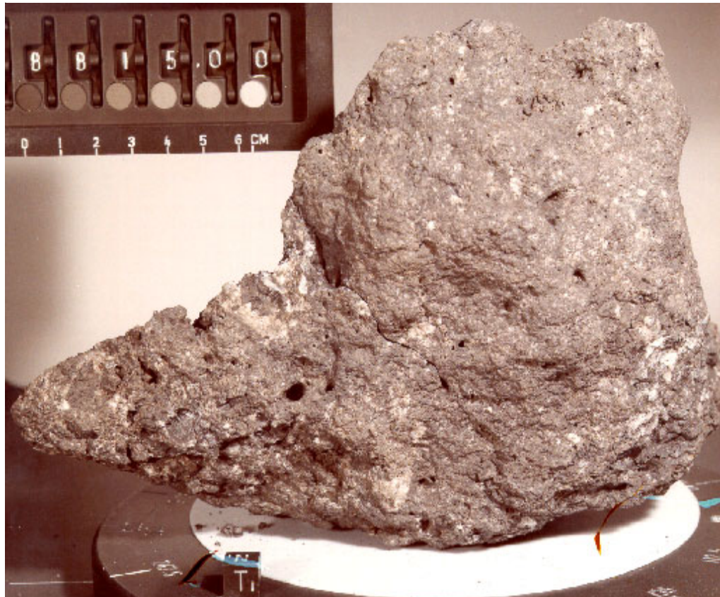
Figure 1: PET photo of 68815, outer surface eroded by zap pits. NASA# S72-37154. Cube is 1 cm.
