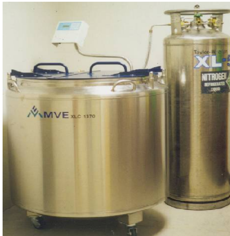
Figure 4. Example of a liquid nitrogen tank used to store Chinook salmon and steelhead gametes.
