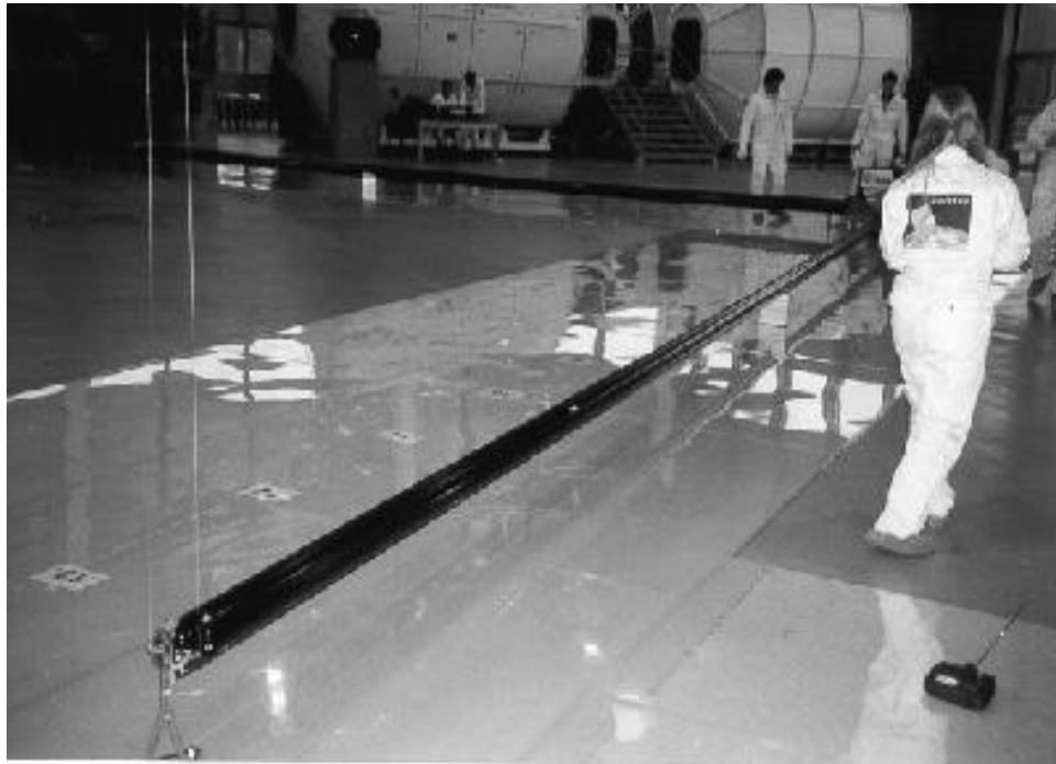
Figure A3 20 x 20 m sail deployment test 17 December – boom deployment
