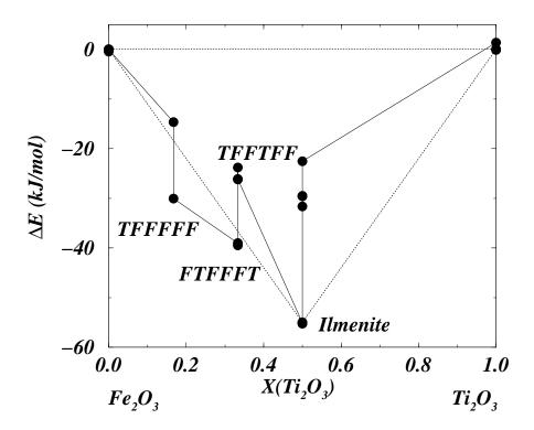
Figure 3: Structure formation energies,  $\Delta E_{Str}$ , for various supercells with bulk compositions that are intermediate between  $\alpha - Fe_2O_3 - FeTiO_3$ .
