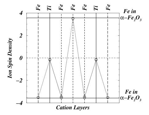
Figure 6: Dmol results for ion spin densities in the FTFFFT... supercell: solid horizontal lines indicate spin densities in  $\alpha-Fe_2O_3$ ; solid vertical lines indicate Ti-layers.
