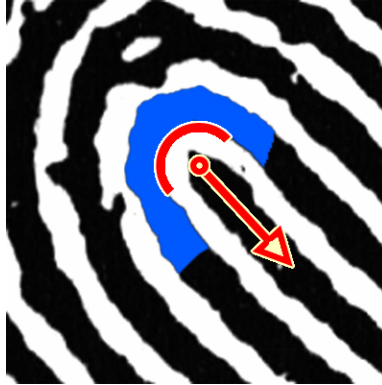
Figure A - 9: Placement of the core at the focus of the innermost recurring ridgeline
