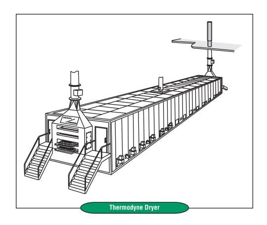
With assistance from the U.S. Department of Energy's Inventions and Innovation Program, Merrill Air Engineers demonstrated that its Thermodyne dryer outperforms conventional molded pulp dryers. Unlike other dryers, the Thermodyne dryer reheats water vapor released from the product being dried to create superheated steam that is directed onto the material being dried. Conventional paper dryers exhaust this liberated water outdoors, causing a large visible plume and dumping valuable heat.
