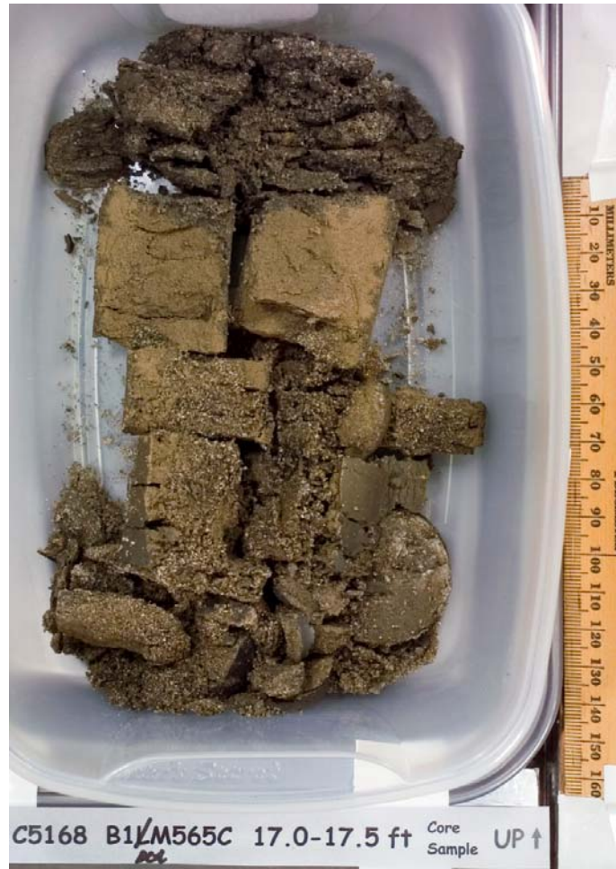
Figure 2.5. Sand-Dominated Sediment Sample from the Hanford Formation H2 Unit. Two medium to coarse sand layers are separated by a thin bed of pale brown very fine sand. Sample collected from push hole C5168 (B Tank Farm), 17.5 to 18.0 ft depth.
