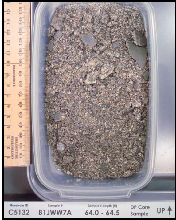
Figure C.5. Sample B1JWW7A from Direct-Push Borehole C5132
