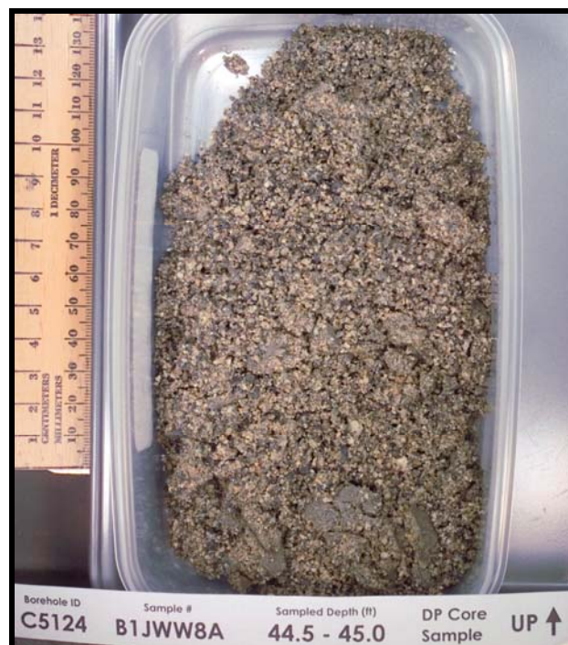
Figure C.2. Sample B1JWW8A from Direct-Push Borehole C5124
