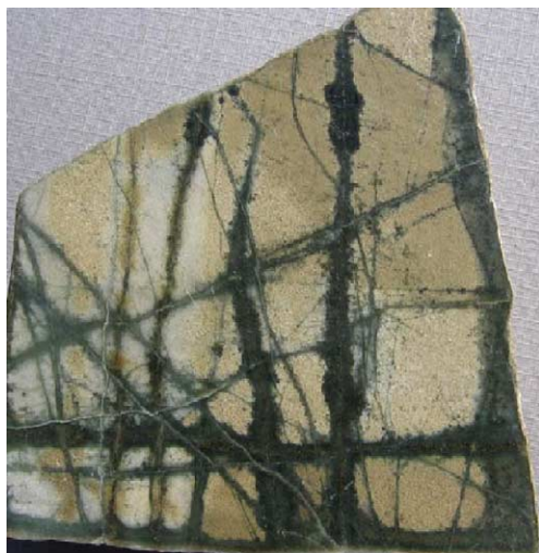
Fig. 5. Example of a reactive fractured rock requiring the use of a hybrid or multiple continuum approach. Actinolite veins (dark green) associated with Fe-metasomatism cutting diopside-rich (tan) rock in the metamorphic aureole of the Bingham porphyry copper deposit. The rock sample is about 10 cm across.
