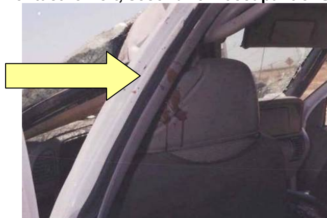
FIGURE 26 Head Contact for left, second row occupant of Suburban
