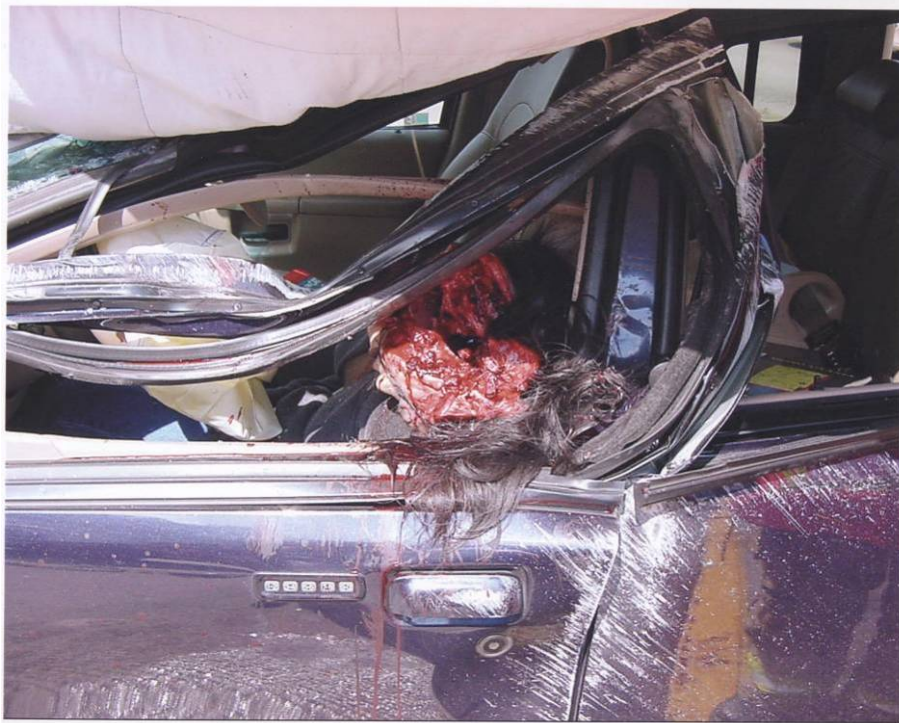
FIGURE 4 Restrained driver's skull cleaved by dynamic, vertical crush of roof rail/window frame
