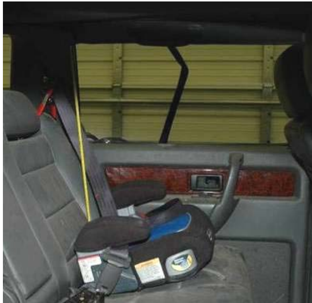
b. Belt positioning booster seat used to restrain the child, according to vehicle and booster seat manufacturer's instructions
