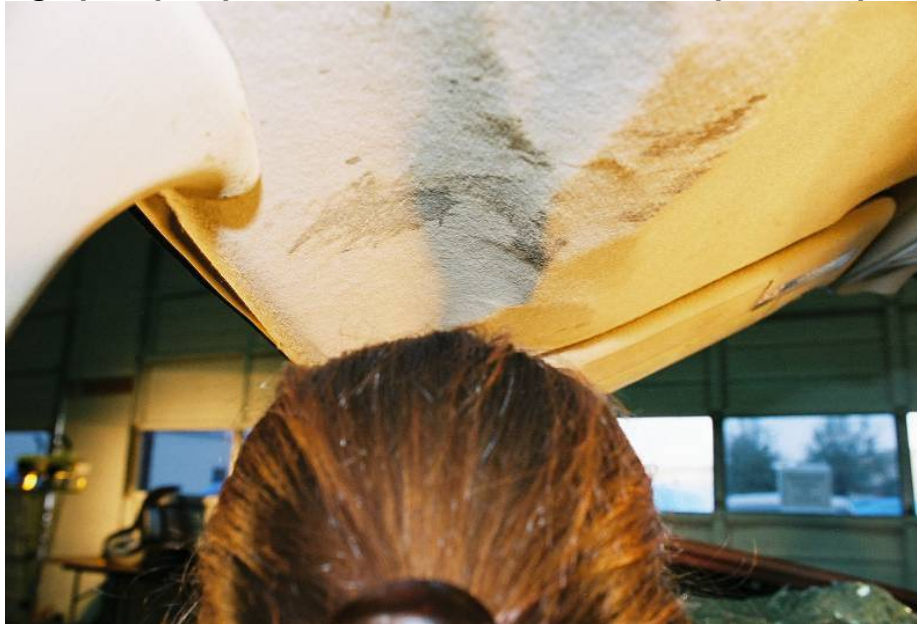
FIGURE 13 Concave Impression in the Driver's Side Roof Liner with Blood Stain (Photographic perspective taken from the rear occupant compartment)
