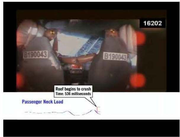
FIGURE 10 Observable Roof Crush and Passenger Neck Load
