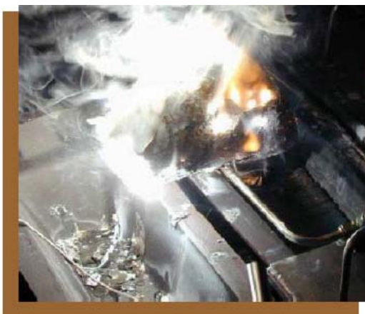
Figure 2. Molten Mg without protective cover gas.
