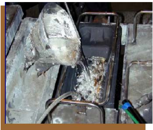
Figure 1. Molten Mg with SF 6 cover gas.
