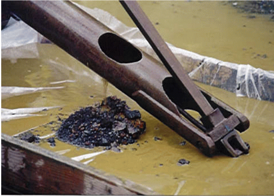
Figure 2. Slag fragments from 11.5 ft bgs removed from borehole MW-206 by the sand pump, November 19, 1997.
