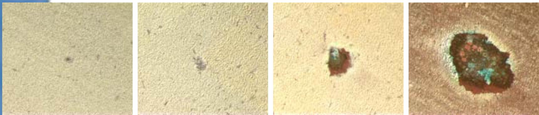
Particle deposition, particle growth, and corrosion cell formation
