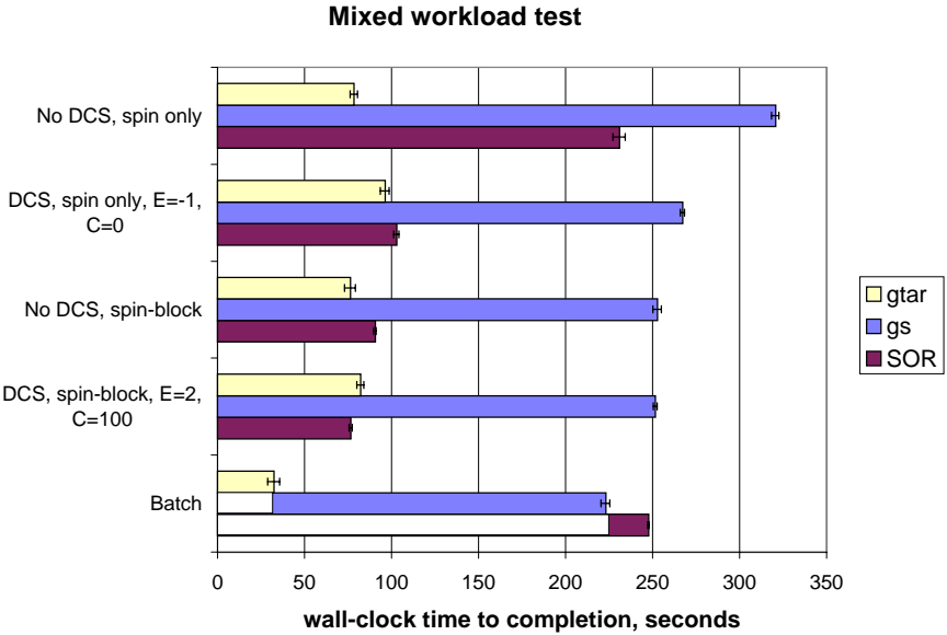
Fig. 11. Job response time in the mixed workload test. In the batch case, jobs were executed in sequence. (N.b.: axes and colors have different significance in these graphs than in the Latency and Barrier results.)
