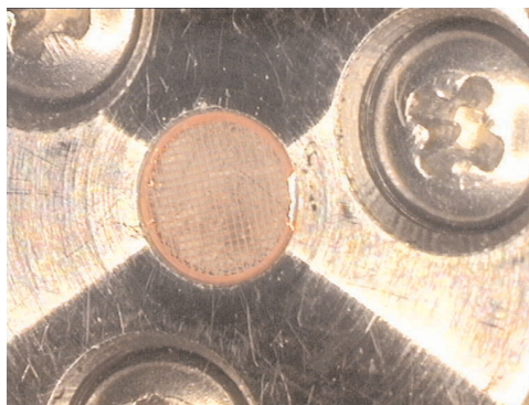
Fig. 4. Image showing the TEM grid placed over the latex membrane within the bubble test fixture prior to Os staining.
