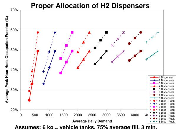
Assumes: 6 kg<sub>H2</sub> vehicle tanks, 75% average fill, 3 min. linger time, 1.67 kg/min hose flow rate
