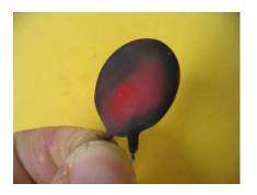
Figure 4 Crispy Factor CF0, indicating an intact MOV covered with soot from other MOVs
