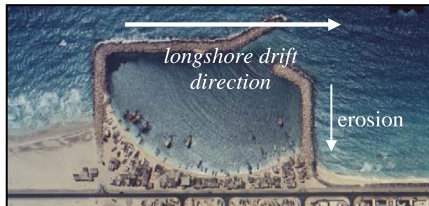
Figure 2: Interruptions of the natural longshore drift of sediment (from south-east to north-west).
