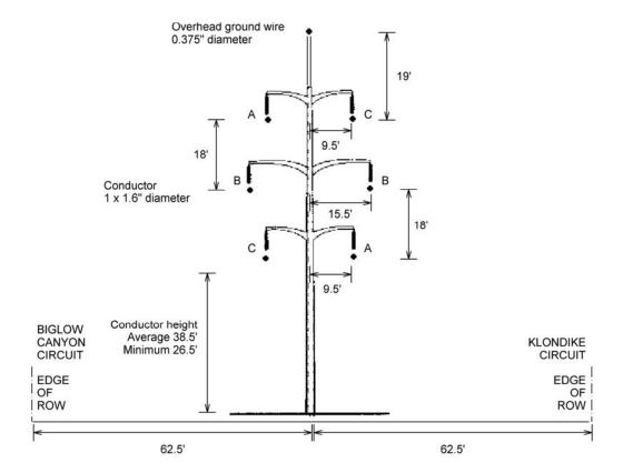
Figure 2: Electric-field profiles for the proposed Klondike – John Day 230-kV transmission line under maximum voltage conditions. Configuration is described in Table 2.
