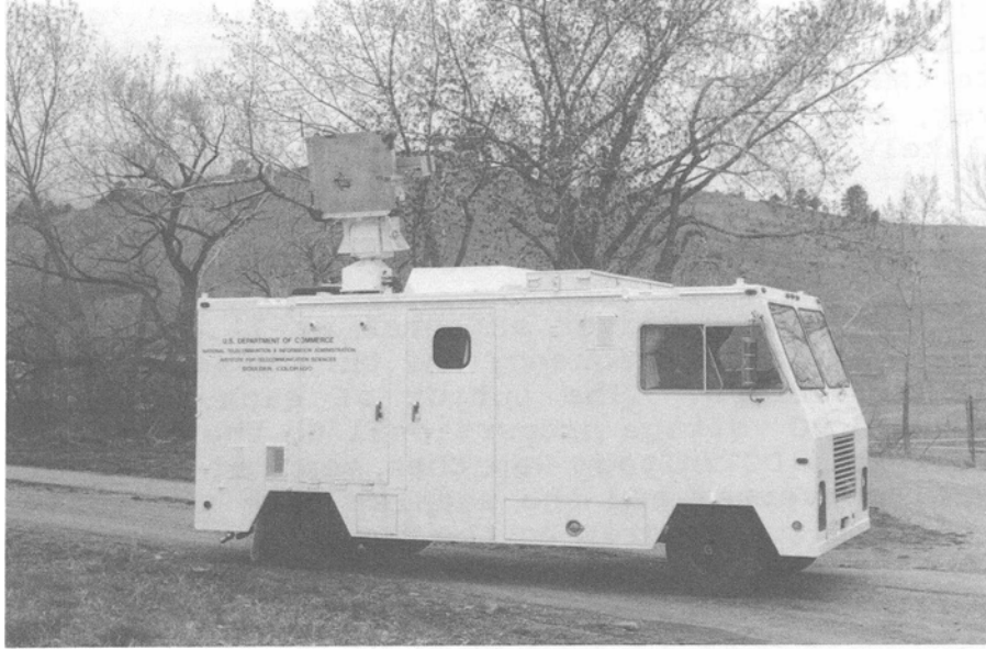
Figure 1. ITS millimeter-wave measurement van (receiver).
