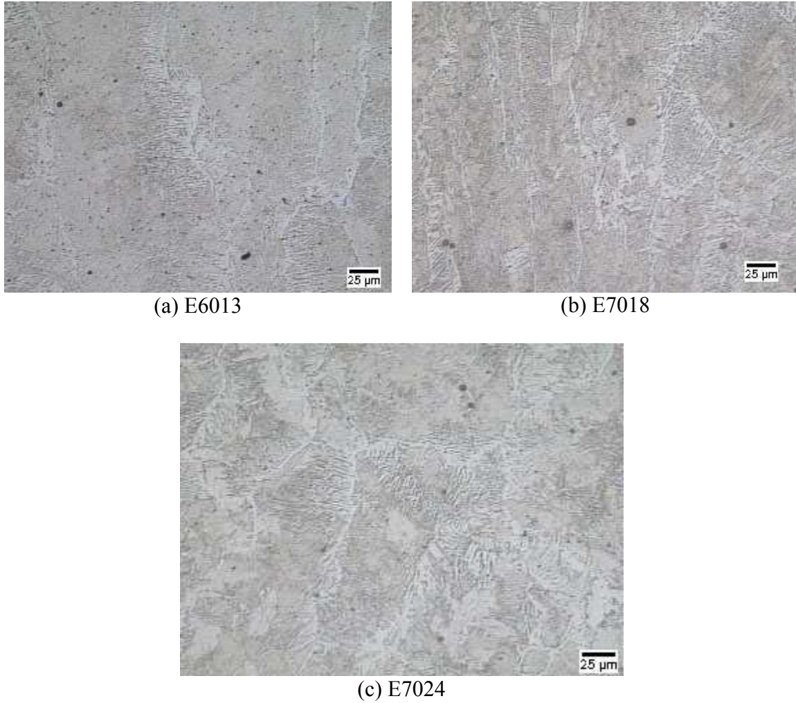
Figure D.1. Microstructures of the bead-on-plate wet welds deposited with the three electrode types using electrode positive on A36 steel at 50 m.
