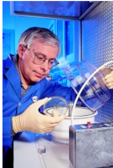
To introduce antifungal genes into barley, biological research technician Robert Campbell places barley tissue into the vacuum pressure chamber of a gene-delivery device.
