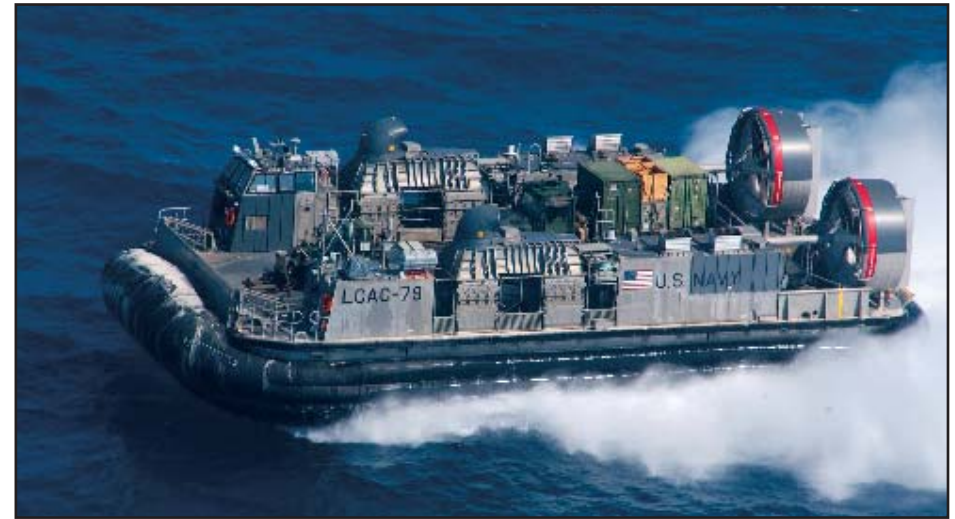
The Landing Craft Air Cushion (LCAC) surface assault ship can carry Marines ashore at speeds in excess of 40 knots.
