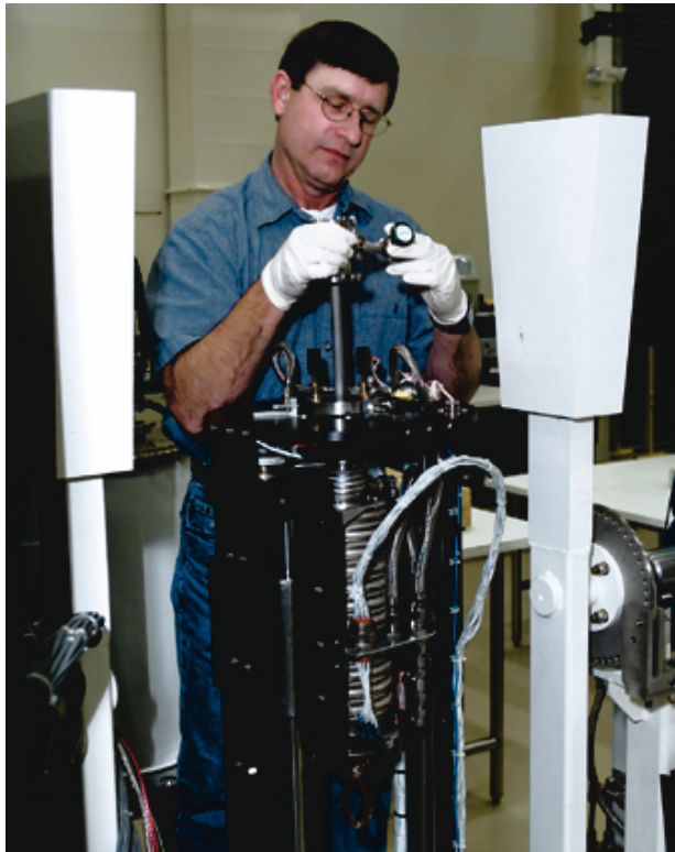
Jeff Dysart, an employee with Ai Signal Research Inc., installs an ampoule into the breadboard furnace.
